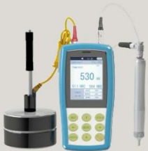
UCL Hardness test using ultra sonic
